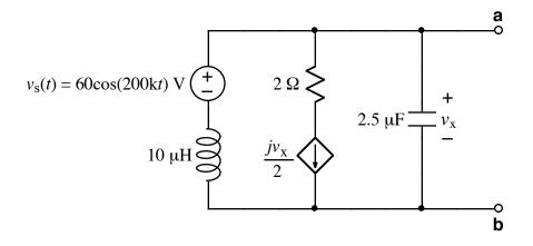
Draw a frequency-domain equivalent of the above circuit. Show a numerical phasor value for  $v_s(t)$ , and show numerical impedance values for R, L, and C. Label the dependent source appropriately.
