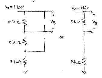
We have a voltage divider:  $v_3 = 10V \cdot 2k\Omega$   $2k\Omega + 3k\Omega$  $V_3 = 4V$
