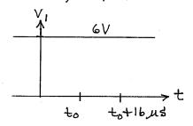
c) From above,  $V_2(0^-) = 6.5V$  and  $V_2(t>0) = 6.5e^{-t/200MS}V$ Also,  $V_2(t=16MS) = V_1 = 6V$
