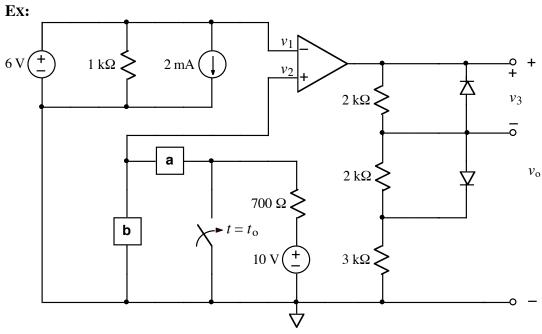
After being open for a long time, the switch closes at time  $t = t_0$ .
