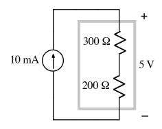
Find the total power dissipated by the components inside the box.
