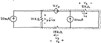
Second, write v-loop egns for loops not containg current src15. There is only one such loop, indicated by the dotted line:
