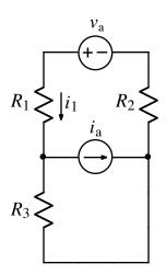
Derive an expression for  $i_1$ . The expression must not contain more than the circuit parameters  $v_a$ ,  $i_a$ ,  $R_1$ ,  $R_2$ , and  $R_3$ .
