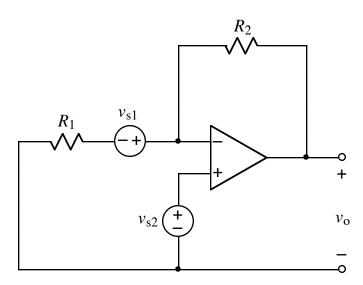
The op-amp operates in the linear mode. Using an appropriate model of the op-amp, derive an expression for  $v_0$  in terms of not more than  $v_{s1}$ ,  $v_{s2}$ ,  $R_1$ , and  $R_2$ .
