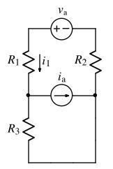
Derive an expression for  $i_1$ . The expression must not contain more than the circuit parameters  $v_a$ ,  $i_a$ ,  $R_1$ ,  $R_2$ , and  $R_3$ .
