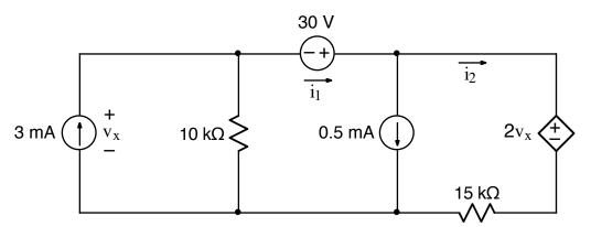
a) Use the mesh-current method to find  $i_1$  and  $i_2$ .
