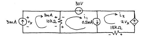
2) We define the voltage from the dependent src, V<sub>X</sub>, in terms of mesh currents. Here, we observe that V<sub>X</sub> is across the 10kΩ resistor, too. For the 10kΩ resistor, we have
