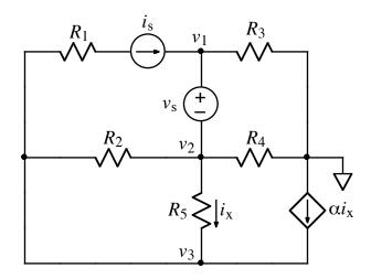
For the circuit shown, write three independent equations for the node-voltages,  $v_1$ ,  $v_2$ , and  $v_3$ . The quantity  $i_x$  must not appear in the equations.
