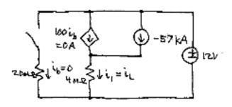
Because of the open circuit on the left, we have  $i_0 = 0$  and  $100i_0 = 0$ .
