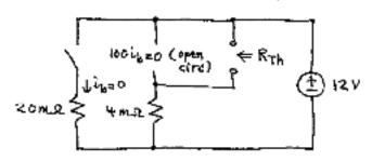
We observe that the Thevenin equivalent seen from the terminals where the L is connected is just the 4ms and 12V:
