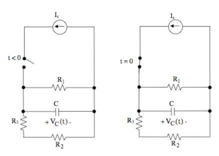
After being open for a long time, the switch closes at t = 0. Write an expression for  $v_C(t > 0)$  in terms of at most circuit quantities  $R_1$ ,  $R_2$ ,  $R_3$ ,  $i_s$ , and C.
