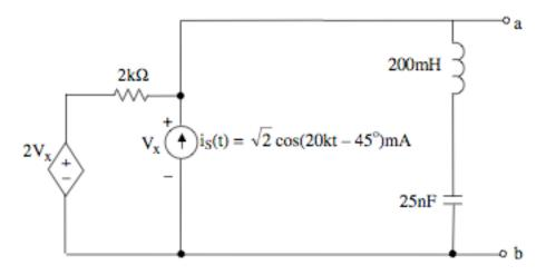
Draw a frequency-domain equivalent of the above circuit. Show a numerical phasor value for  $i_s(t)$ , and show numerical impedance values for R, L, and C. Label the dependent source appropriately.
