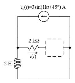
Choose an *R*, an *L*, or a *C* to be placed in the dashed-line box to make  $i(t) = I_0 \cos(1kt + 45^\circ)$
