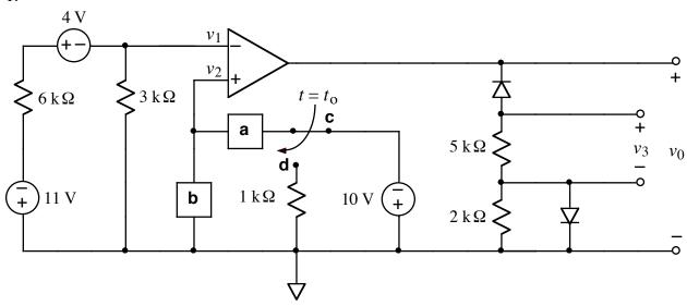
After being in position **c** for a long time, the switch moves from **c** to **d** at  $t = t_0$ . Rail voltages =  $\pm 12$  V
