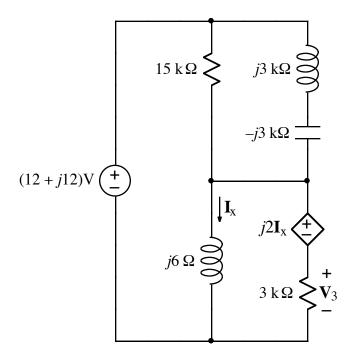
A frequency-domain circuit is shown above. Write the value of phasor  $\mathbf{V}_3$  in polar form.
