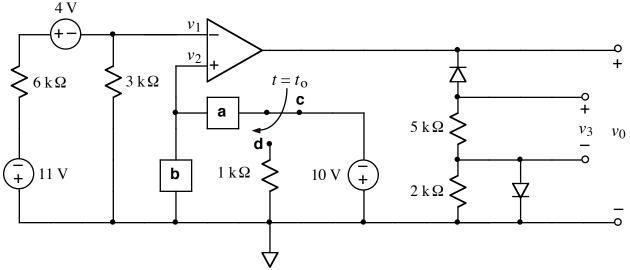
After being in position **c** for a long time, the switch moves from **c** to **d** at  $t = t_0$ . Rail voltages = ±12 V
