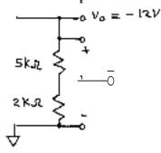
We have a voltage divider:  $v_3 = -12 \text{ V} \cdot \frac{5 \text{ k}\Omega}{2 \text{ k}\Omega + 5 \text{ k}\Omega} = -\frac{60}{7} \text{ V}.$
