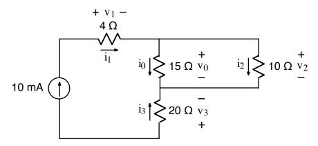
In general, measuring the voltage with the + sign on the top or on the left side proves to be convenient.
