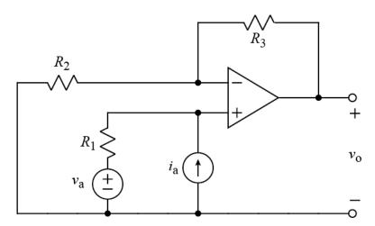
The op-amp operates in the linear mode. Using an appropriate model of the op-amp, derive an expression for  $v_0$  in terms of not more than  $v_a$ ,  $i_a$ ,  $R_1$ ,  $R_2$ , and  $R_3$ .
