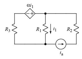
Derive an expression for  $i_1$ . The expression must contain no other parameters than  $i_a$ ,  $R_1$ ,  $R_2$ ,  $R_3$ , and  $\alpha$ . **Note:**  $\alpha < 0$ . (Hint: It is not just a voltage or current divider.)
