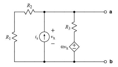
Find the Thevenin equivalent circuit at terminals a-b.  $v_x$  must not appear in your solution. The expression must not contain more than circuit parameters  $\alpha$ ,  $R_1$ ,  $R_2$ ,  $R_3$ , and  $i_s$ . **Note:**  $0 < \alpha < 1$ .
