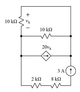
Calculate the power dissipated by the dependent current source, (labeled  $20v_x$ ).
