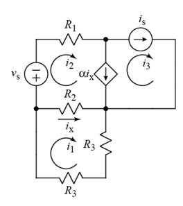
For the circuit shown, write three independent equations for the three mesh currents,  $i_1$ ,  $i_2$ , and  $i_3$ . The quantity  $i_x$  must not appear in the equations.
