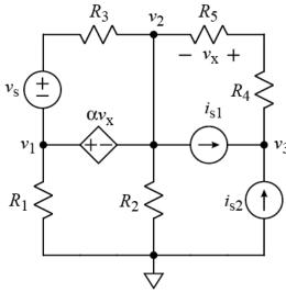
For the circuit shown, write three independent equations for the node-voltages,  $v_1$ ,  $v_2$ , and  $v_3$ . The quantity  $v_x$  must not appear in the equations. Only component and source names may appear in answer.
