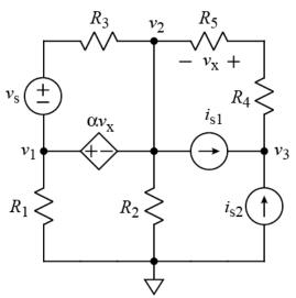
For the circuit shown, start with three independent equations for the node-voltages,  $v_1$ ,  $v_2$ , and  $v_3$ . The quantity  $v_x$  must not appear in the equations. Only component and source names may appear in answer.
