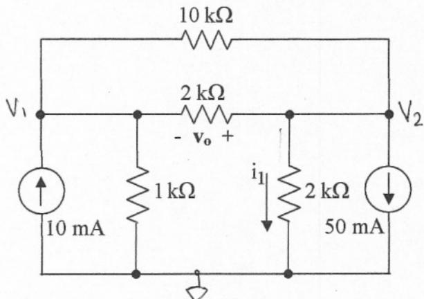
$$V_o = (V_2 - V_1) = -52.86 + 13.6 = \boxed{-39.26 \text{ V}}$$
