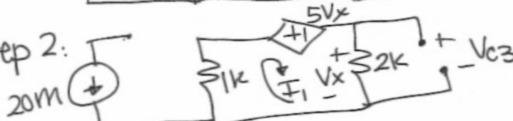
$\gamma \Rightarrow$  since  $V_{c3}=0$ , need to use test source
