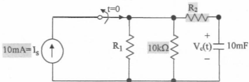
After being closed for a long time, the switch becomes open at  $t=0$ . Find  $R_1$  and  $R_2$  that give the following plot for  $V_c(t)$ :
