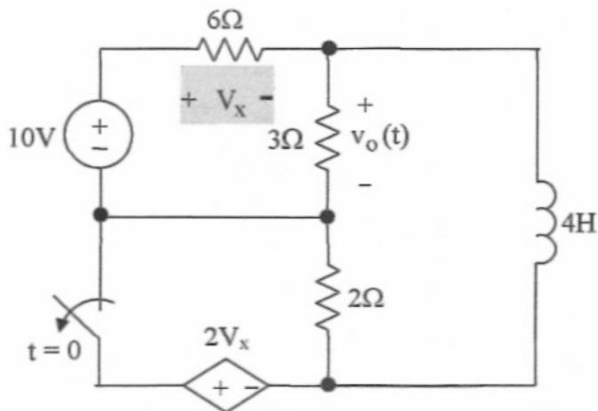
After the switch has been closed for a long time, it opens at  $t=0$ . Find the output voltage  $v_o(t)$  for  $t > 0$ .
