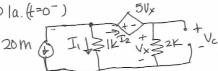
$$\Sigma I: +20m + I_1 + I_2 = 0 \Rightarrow I_1 = (-I_2 - 20m)$$
