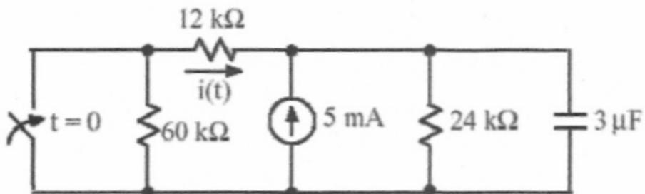
Step 1: After being open for a long time, the switch becomes closed at  $t=0$ . Find  $i(t)$  for  $t > 0$ .
