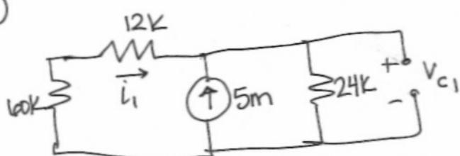
$$V_{C1} = \left[ \frac{5m(72k)}{72k+24k} \right] 24k = 90V$$
