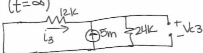
$$V_{C3} = \left[ \frac{5m(12k)}{12k+24k} \right] 24k = 40V$$
