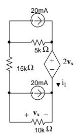
Find  $v_x$ ,  $i_1$ , and the power dissipated by the dependent source.
