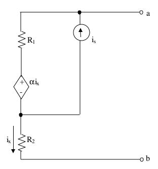
Find the Thevenin equivalent circuit at terminals a-b.  $i_x$  must not appear in your solution. **Note:** 0 < a < 1.
