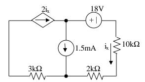
Calculate the power consumed (ie dissipated) by the 18V source. **Note:** If a source supplies power, the power it consumes is negative.
