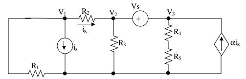
For the circuit shown, write three independent equations for the node voltages  $V_1$ ,  $V_2$ , and  $V_3$ . The quantity  $i_x$  must not appear in the equations.
