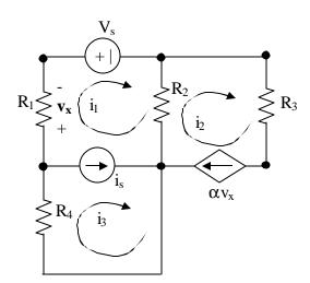
For the circuit shown, write three independent equations for the three mesh currents  $i_1$ ,  $i_2$ , and  $i_3$ . The quantity  $v_x$  must not appear in the equations.
