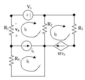
For the circuit shown, write three independent equations for the three mesh currents  $i_1$ ,  $i_2$ , and  $i_3$ . The quantity  $v_x$  must not appear in the equations.
