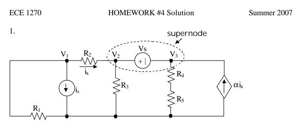
For the circuit shown, write three independent equations for the node voltages  $V_1$ ,  $V_2$ , and  $V_3$ . The quantity  $i_x$  must not appear in the equations.
