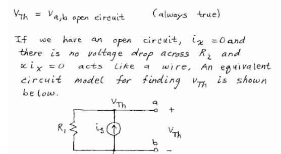
We see by inspection that  $v_{Th}$  is across  $R_1$  and  $V_{Th} = i_{\beta}R_1$  by Ohm's law.
