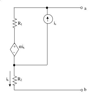
Find the Thevenin equivalent circuit at terminals a-b.  $i_x$  must not appear in your solution. Note: 0 < a < 1.
