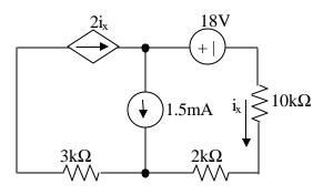
Calculate the power consumed (ie dissipated) by the 18V source. **Note:** If a source supplies power, the power it consumes is negative.
