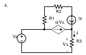
Using superposition, derive an expression for i that contains no circuit quantities other than Is, Vs, R1, R2, R3, and  $\alpha$ , where  $\alpha$ >0.
