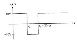
Choose either an R or C to go in box  $\mathbf{a}$  and either an R or L to go in box  $\mathbf{b}$  to produce the  $v_0(t)$  shown above. Use an R value of 3 k $\Omega$ . Also, note that  $v_0$  stays high forever after  $t_0 + 20 \,\mu s$ . Specify which element goes in each box and its value.
