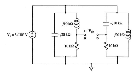
A frequency-domain circuit is shown above. Write the value of phasor voltage  $\mathbf{V}_{ab}$  in polar form.
