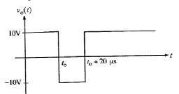
Choose either an R or C to go in box **a** and either an R or L to go in box **b** to produce the  $v_0(t)$  shown above. Use an R value of 3 k $\Omega$ . Also, note that  $v_0$  stays high forever after  $t_0 + 20 \,\mu$ s. Specify which element goes in each box and its value.
