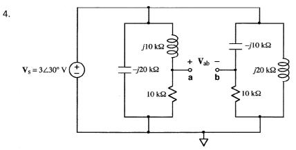
A frequency-domain circuit is shown above. Write the value of phasor voltage  $\mathbf{V}_{ab}$  in polar form.
