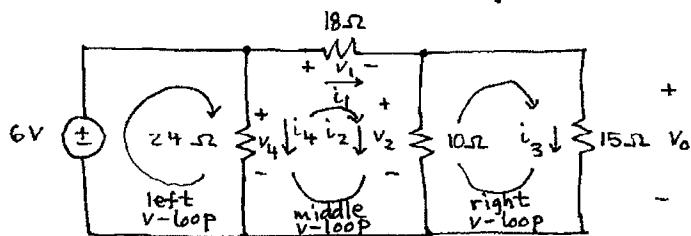
Write eqns for voltage loops for inner loops
