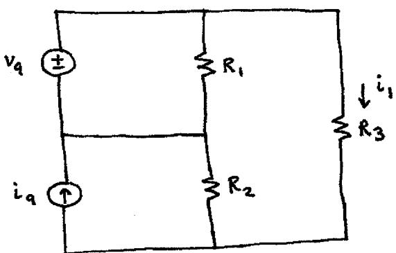
Derive expression for  $i_1$ . Expression must contain no other parameters than  $V_a$ ,  $i_a$ ,  $R_1$ ,  $R_2$ ,  $R_3$ .
