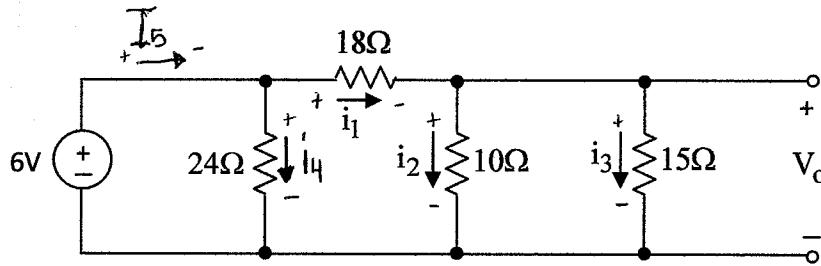
$$\text{KVL: } +6 - i_4(24) = 0 \Rightarrow i_4 = \frac{6}{24} = 250 \text{ mA}$$
