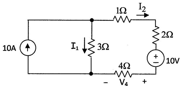
$$V_4 = 8V = I_2 \cdot 4\Omega \Rightarrow I_2 = 8/4\Omega = \boxed{2A}$$
