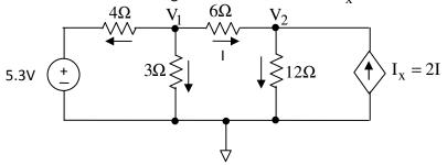
Using the bottom node as the reference node, two equations stated below are determined by setting the sum of currents(directions as shown) out each node equal to zero.
