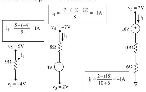
To determine the signs, if we were to mark a + and – for a voltage measurement across the 9  $\Omega$  resistor that is in the passive sign direction for  $i_1$ , then we add  $v_2$  (which is next to the + sign) and subtract  $v_1$  (which is next to the – sign).
