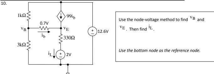
Sol'n: Write current summations for  $v_B$  and  $v_E$  nodes. The second equation is the supernode equation. The first equation is due to a supernode between  $v_B$  and  $v_E$
