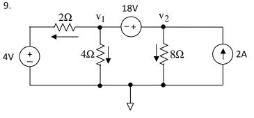
Use the node-voltage method to find  $\,v_1\,$  and  $\,v_2\,.$
