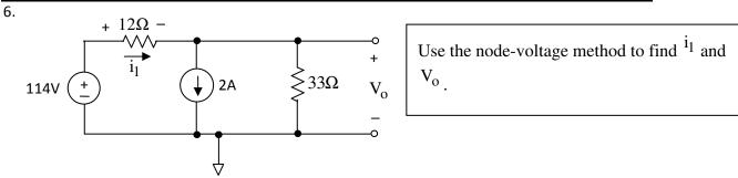
Set the reference point at the bottom node and Vo as the top node. We set the sum of currents out of v1 equal to zero, group terms for Vo and then solve:
