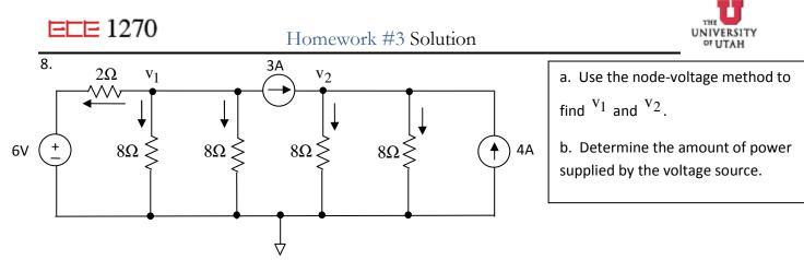
(a) We derive two equations by setting the sum of currents out each node equal to zero.
