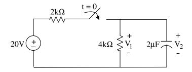
3. After being open for a long time, the switch closes at t = 0. Find  $i_1(t)$  for t > 0.
