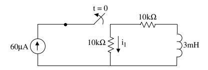
2. After being open for a long time, the switch closes at t = 0. Find  $V_1(t)$  for t > 0.
