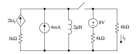
4. After being open for a long time, the switch closes at t = 0. Find  $i_1(t)$  for t > 0.
