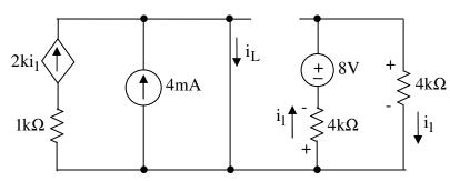
When the circuit contains a dependent source, an extra step is needed to determine the value of the dependent variable:
