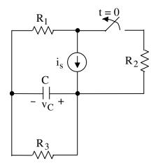
SOL'N: a) We first find the voltage across the capacitor for  $t = 0^-$ . The switch is open, eliminating  $R_2$  from consideration. The capacitor looks like an open. This leaves only the  $i_8$  source driving  $R_1$  and  $R_3$  in series. The capacitor is directly across  $R_3$  and so has the same voltage as  $R_3$ :
