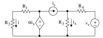
SOL'N: First, we turn off the independent source,  $i_s$ . This means the current source turns into an open circuit, separating the circuit into two pieces. On the right, we have  $v_s$  in series with  $R_3$  and  $R_4$ .
