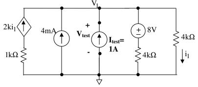
To find  $R_{eq}$  the inductor is removed from the final circuit to find path from top of inductor to bottom of inductor(Thevenin Resistance):
