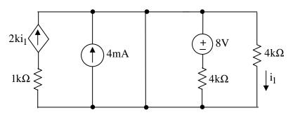
This wire puts 0V across 4k ohm resistor so:  $i_1$ =0
