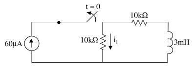
Step 1: (Redraw circuit at t=0 and solve for  $i_L$ . Inductor acts as a wire since it has sat for a long time)
