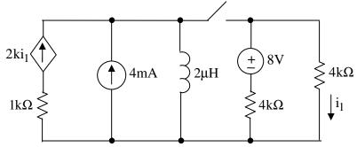
Step 1: (Redraw circuit at **t=0** and solve for i<sub>L</sub>. Inductor acts as a wire since it has sat for a long time)
