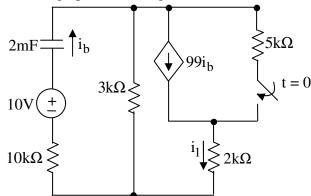
Step 1: (Redraw circuit at **t=0** and solve for V<sub>C</sub>. Capacitor acts as an open since it has been a long time)
