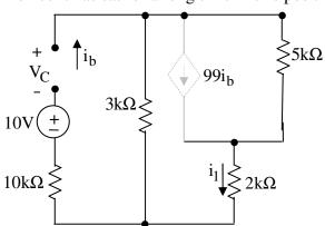
this means that 99ib source becomes open.  $i_b=0$
