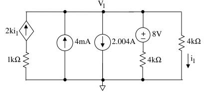
Solve the circuit for  $i_1$ . Mesh currents or node-voltage can be used. Node-voltage method:
