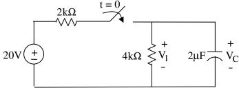
Step 1: (Redraw circuit at t=0 and solve for  $V_C$ . Capacitor acts as an open since it has been a long time)
