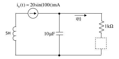
a. Choose an R, an L, or a C to be placed in the dashed-line box to make
