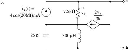
Draw a frequency-domain equivalent of the above circuit. Show a numerical phasor value for  $i_s(t)$ , and show numerical impedance values for R, L, and C. Label the dependent source appropriately.
