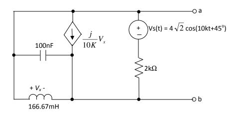
a) Draw a frequency-domain equivalent of the above circuit. Show a numerical phasor value for  $V_S(t)$ , and show numerical impedance values for R, L, and C. Label the dependent source appropriately.
