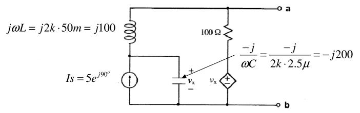
8. Find the Thevenin equivalent (in the frequency domain) for the circuit from Problem 8. Give the numerical phasor value for  $\,V_{Th}\,$  and the numerical impedance value of  $\,z_{Th}$ .
