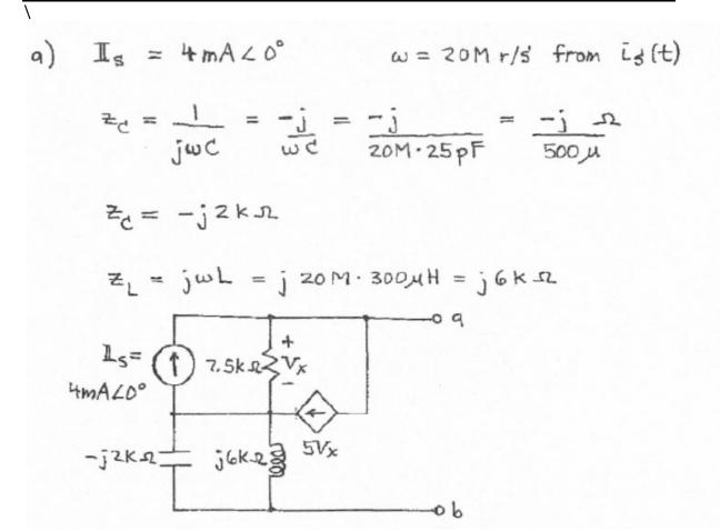
6. Find the Thevenin equivalent (in the frequency domain) for the circuit from Problem 6. Give the numerical phasor value for  $V_{Th}$  and the numerical impedance value of  $z_{Th}$ .
