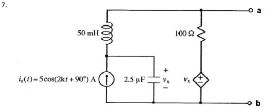
Draw a frequency-domain equivalent of the above circuit. Show a numerical phasor value for  $i_s(t)$ , and show numerical impedance values for R, L, and C. Label the dependent source appropriately.
