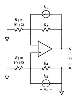
The above circuit operates in linear mode. Derive a symbolic expression for  $v_0$ . The expression must contain not more than the parameters  $i_{s1}$ ,  $i_{s2}$ ,  $R_1$ ,  $R_2$ ,  $R_3$ , and  $R_4$ .
