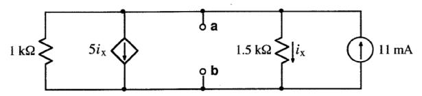
Find the Thevenin equivalent of the above circuit relative to terminals a and b.
