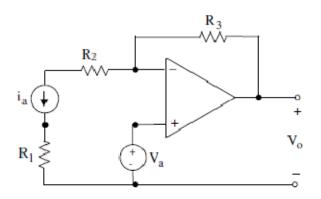
The op-amp operates in the linear mode. Using an appropriate model of the opamp, derive an expression for  $V_0$  in terms of not more than  $i_a$ ,  $R_1$ ,  $R_2$ ,  $R_3$ , and  $V_a$ .
