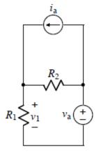
Derive an expression for  $v_1$ . The expression must not contain more than the circuit parameters  $i_a$ ,  $v_a$ ,  $R_1$ , and  $R_2$ .
