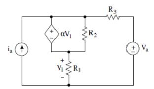
) Derive the expression for  $V_1$  containing not more than circuit parameters  $\alpha,\,R_1,\,R_2,\,R_3,\,V_a,\,and\,i_a.$
