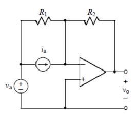
The op-amp operates in the linear mode. Using an appropriate model of the opamp, derive an expression for  $v_0$  in terms of not more than  $i_a$ ,  $v_a$ ,  $R_1$ , and  $R_2$ .
