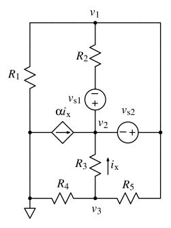
For the circuit shown, write three independent equations for the node voltages  $v_1$ ,  $v_2$ , and  $v_3$ . The quantity  $i_X$  must not appear in the equations.
