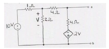
5. Determine the power in the dependent source if  $R_L$  =2k $\!\Omega$
