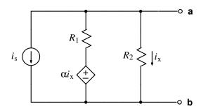
Find the Thevenin equivalent circuit at terminals **a** and **b**.  $i_X$  must not appear in your solution. **Note:**  $\alpha > 0$ .
