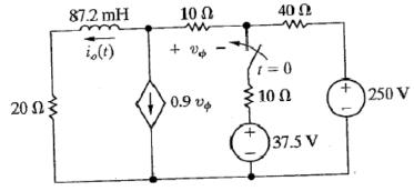
4. After being closed for a long time, the switch opens at t = 0. Find  $i_b(t)$  for t > 0.
