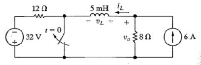
2. After being open for a long time, the switch closes at t = 0. Find  $i_1(t)$  and  $i_2(t)$  for t > 0.
