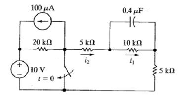
3. After being open for a long time, the switch closes at t = 0. Find  $v_{\phi}(t)$  for t > 0.
