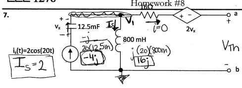
Draw a frequency-domain equivalent of the above circuit. Show a numerical phasor value for  $i_s(t)$  , and show numerical impedance values for R, L, and C. Label the dependent source appropriately.
