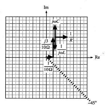
The solution for  $1/z_{box}$  must be an inductor that moves the total down to 1
