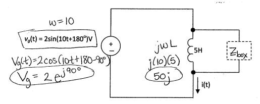
Choose an R, an L, or a C to be placed in the dashed-line box to make  $(i(t) = I_0 \cos(10t+45^\circ)A)$ where  $\mathbf{I}_{\mathbf{0}}$  is a real constant. State the value of the component you choose.
