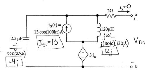
Draw a frequency-domain equivalent of the above circuit. Show a numerical phasor value for  $i_{\rm S}(t)$ , and show numerical impedance values for R, L, and C. Label the dependent source appropriately.
