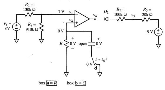
The output of the op-amp will switch from high to low when the op-amp input voltages are equal:  $v_2 = v_1 = 7$  V. The value of C is chosen to cause switching at time  $t_0 + 25$   $\mu$ s using the formula  $v_2(t)$ .
