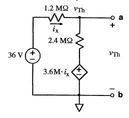
First, we define the dependent variable,  $i_x$ , in terms on node voltage  $v_{Th}$ .
