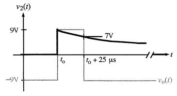
When  $v_0$  is low, the current will try to flow from right (where the +9 V supply is located) to the left (where  $v_0 = -9$  V). The diode is forward biased in this case and allows the current to flow. (The diode allows current to flow in the direction of the "arrow" in the diode symbol.) The diode acts like a wire and  $R_3$  and  $R_5$  form a voltage-divider. There are
