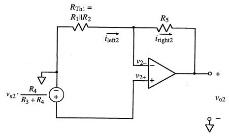
For this circuit,  $v_{2-} = v_{2+} = v_{s2} \frac{R_4}{R_3 + R_4}$ . (The "2" stands for "case II".)
