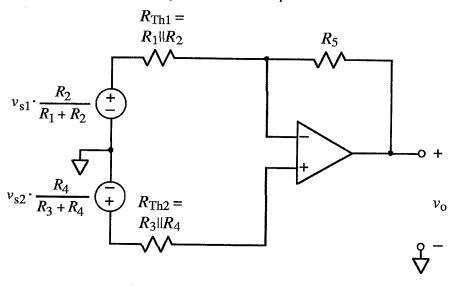
Since no current flows into the + input of the op-amp,  $R_{Th2}$  has no voltage drop and may be removed.
