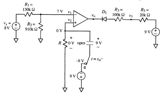
At time  $t = 0^+$ , the voltage across the capacitor remains the same, namely 9 V. As shown below,  $v_2$  will jump up to 9 V. This means  $v_2 = 9 \text{ V} > v_1 = 7 \text{ V}$  and  $v_0 = -v_{\text{rail}}$ , as desired in the problem. This is a satisfactory configuration for initial conditions.
