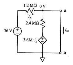
The current contributed to  $i_{\rm sc}$  by the dependent source is given by the voltage loop on the right:
