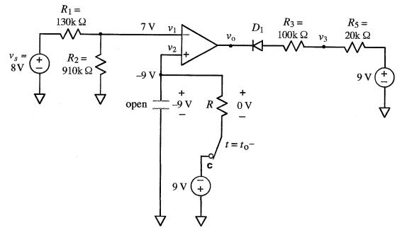
At time  $t = 0^+$ , however, the voltage across the capacitor and voltage  $v_2$  remain the same, namely -9 V. Thus,  $v_0$  would not immediately change to  $+v_{\rm rail}$  as required in the statement of the problem, and this is an incorrect configuration.
