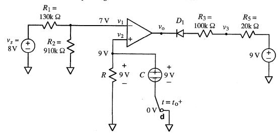
The next step is to examine the final conditions in the circuit, to determine whether  $v_2 < v_1 = 7$  V as time approaches infinity so that  $v_0$  will be negative as time approaches infinity. As shown in the diagram below,  $v_2$  will fall to 0 V, thus yielding the appropriate circuit behavior. Thus, this circuit can satisfy the problem requirements.
