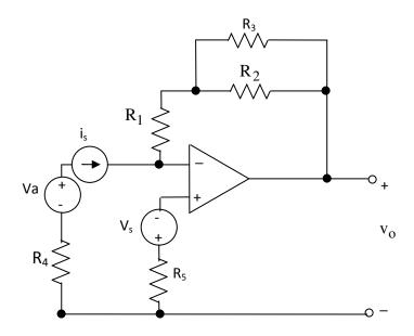
9. The op-amp operates in the linear mode. Using an appropriate model of the op-amp, derive an expression for Vo in terms of not more than i<sub>a</sub>, R1, R2, R3, and/or Va. Note that the current source is **not** ideal and has a voltage drop across it.
