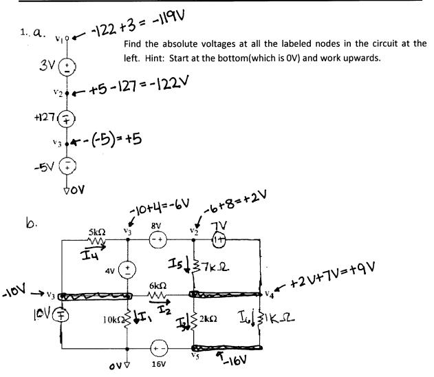
Find the absolute voltages at all the labeled nodes in the above circuit. Hint: This may be done by inspection.
