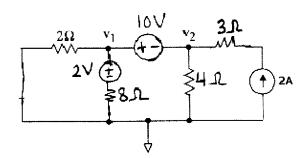
Use either the node-voltage method or current mesh method to find  $\,v_1\,$  and  $\,v_2\,.$
