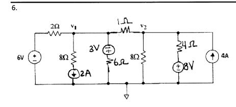
a. Use the node-voltage method to find  $\,v_1\,$  and  $\,v_2\,.$
