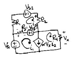
Use the mesh-current method to find  $\,i_1$  and  $\,i_2$  , and  $\,i_3$  .
