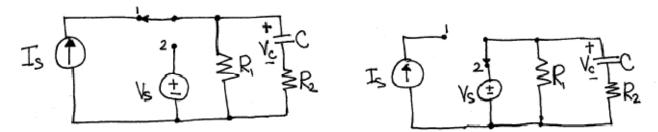
After being in position 1(left circuit) for a long time, the switch moves to position 2 at t=0(right circuit).
