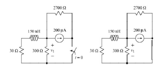
After being open(left circuit) for a long time, the switch closes at t = 0(right circuit).
