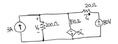
Using superposition, derive a value for  $i_{1}$ .
