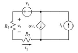
Using superposition, derive an expression for  $i_1$  that contains no circuit quantities other than  $i_s$ ,  $v_s$ ,  $R_1$ ,  $R_2$ , and  $\alpha$ . Note:  $\alpha > 0$ .
