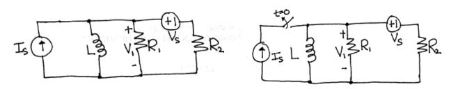
After being closed(left circuit) for a long time, the switch opens at t = 0(right circuit).
