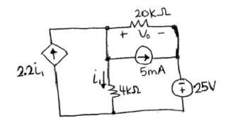
Using superposition, derive an expression for  $V_0$ .
