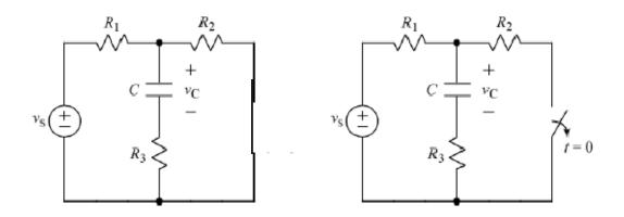
After being closed(left circuit) for a long time, the switch opens at t = 0(right circuit).
