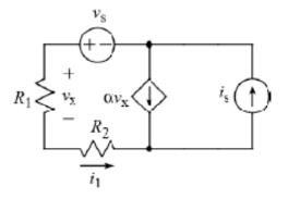
Using superposition, derive an expression for  $i_1$  that contains no circuit quantities other than  $i_s$ ,  $v_s$ ,  $R_1$ ,  $R_2$ , and  $\alpha$ . Note:  $\alpha > 0$ .
