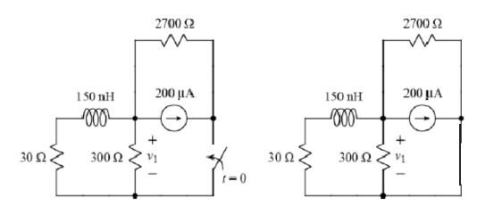
After being open(left circuit) for a long time, the switch closes at t = 0(right circuit).
