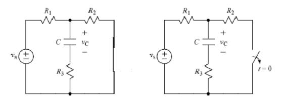
After being closed(left circuit) for a long time, the switch opens at t = 0(right circuit).
