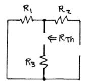
Because the switch is open, Rz has no effect on R<sub>Th</sub>. Since R, and R<sub>3</sub> are in series, we have
