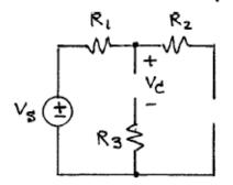
With the open circuits, no durrent Flows. Thus, the v-drops for the R's are zero. For the v-loop on the left, we have
