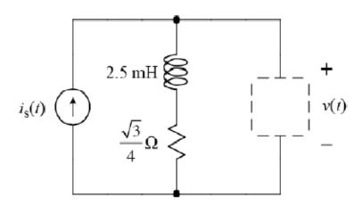
a) The current source in the above circuit has a value of  $i_s(t) = 4\cos(100t)$  A
