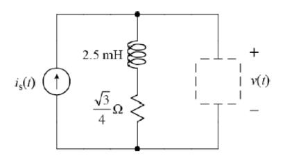
a) The current source in the above circuit has a value of  $i_s(t) = 4\cos(100 t) A$
