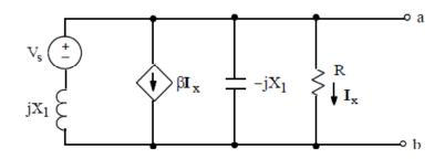
Construct a frequency-domain Thevenin equivalent circuit with respect to terminals a-b. Note that the L and C have impedances with equal magnitudes but opposite signs. Also,  $\mathbf{I}_{\mathbf{x}}$  must <u>not</u> appear in your answer.
