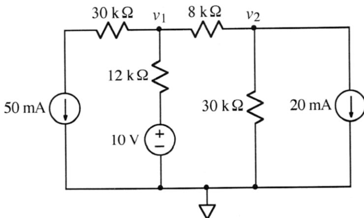
Use the node-voltage method to find  $v_1$  and  $v_2$ .
