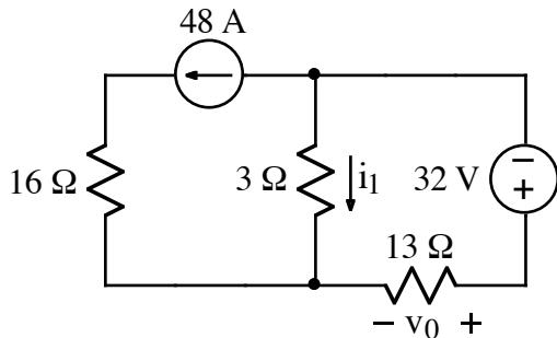
Use the node-voltage method to find  $i_1$  and  $v_0$ .sol'n: We sum currents out of  $v_1$  node:
