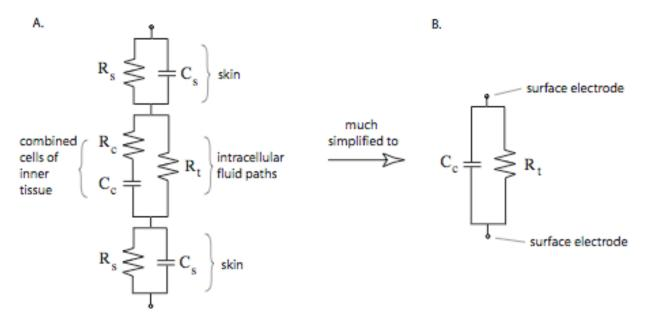
Fig. 2 – A) Lumped-element model of the electrical behavior of tissue bordered by skin, B) After several simplifications, the model reduces to its essence, a parallel *RC* circuit.
