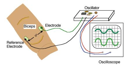
Figure 5. Tissue measurement configuration.
