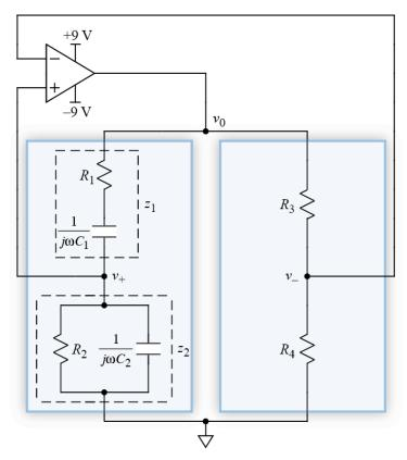
Figure 4. Wien-bridge oscillator schematic. Shaded boxes indicate voltage dividers.
