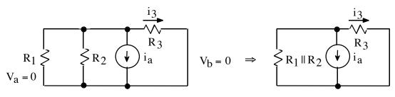
By current divider formula, we have  $i_3 = -\frac{i_a R_1 || R_2}{R_1 || R_2 + R_3}$ .
