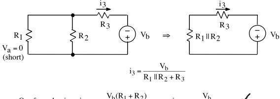
Our formula gives  $i_3 = \frac{V_b(R_1 + R_2)}{R_1R_2 + R_3(R_1 + R_2)}$  or  $i_3 = \frac{V_b}{R_1 ||R_2 + R_3}$ .
