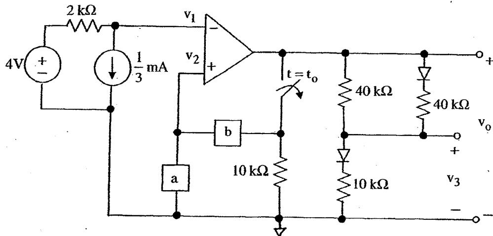
Rail voltages =  $\pm 10$  VAfter being closed for a long time, the switch closes at  $t = t_0$ .
