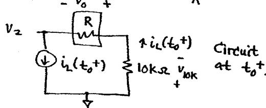
At  $t_0^+$ , the current in R will be  $i_L(t_0^+) = i_L(t_0^-) = \frac{v_o}{R}$  or the same as at  $t_0^-$ . Thus, the v-drop for R at  $t_0^+$  will be  $v_o$ . Current  $i_L(t_0^+)$  flowing in the  $10k\Omega$  will cause a voltage drop in series with the drop for R, resulting in a very negative voltage at  $v_2$ . This would cause  $v_o$  to go low at  $t = t_0^+$  rather than after a delay of 5  $\mu s$ .
