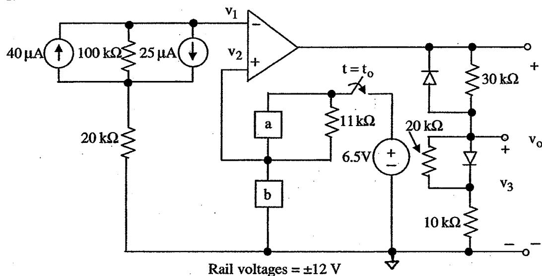
After being open for a long time, the switch closes at  $t = t_0$ .
