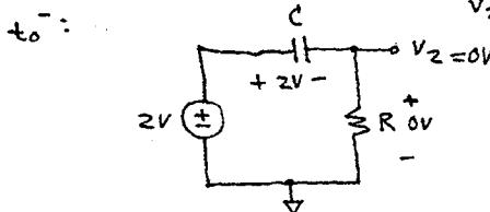
When switch closes,  $v_C$  will stay at  $2V$  for  $t=t_0^+$ :
