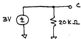
$$V_{Th} = 3V \text{ since } C \text{ connected to } 3V \text{ source}$$
