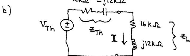
$$P = (\text{ave pwr in } Z_L) = \frac{|I|^2}{2} R \text{ where } R = 16k\Omega \text{ in } Z_L$$
