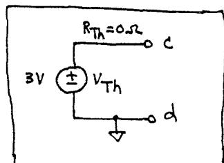
$$R_{Th} = R \text{ looking into } C \text{ with } 3V \text{ source shorted}$$
