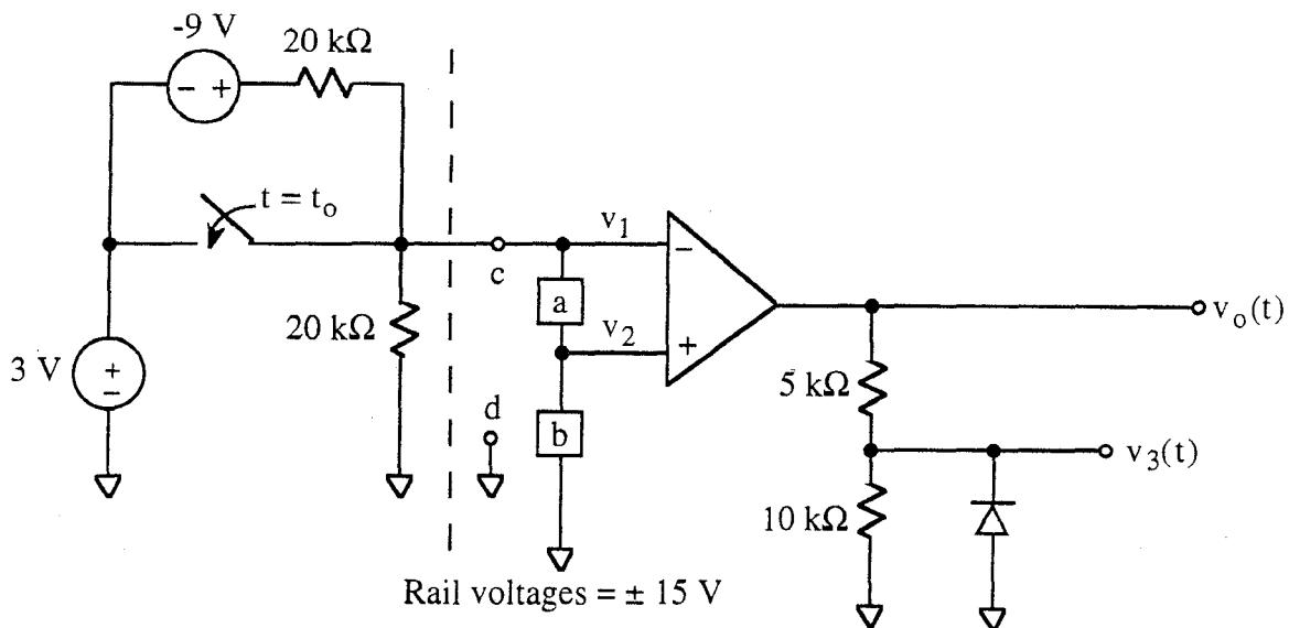
After being open for a very long time, the switch closes at  $t = t_0$ .
