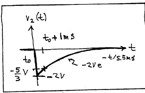
$$\begin{aligned} \text{Let } t_0 &= 0 & -t/RC \\ v_2(t) &= -2V e^{-t/RC} \\ v_2(1\text{ms}) &= -2V e^{-1\text{ms}/RC} = -\frac{5}{3}V \\ e^{-1\text{ms}/RC} &= \frac{5}{6} \end{aligned}$$
