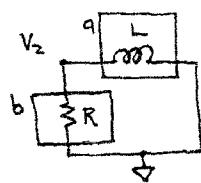
$$\begin{aligned} v_2(t > 0) &= v_2(t \rightarrow \infty) + [v_2(0^+) - v_2(t \rightarrow \infty)] e^{-t/\tau} \\ &= 0V + [v_2(0^+) - 0V] e^{-t/\tau} \\ &= v_2(0^+) e^{-t/\tau}; \text{ Now find } v_2(0^+). \end{aligned}$$
