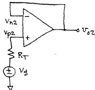
$$v_{p2} = v_s \text{ (no current in } R_T \text{ so no V-drop)}$$
