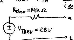
Sol'n: 3.b) Max pwr when  $R_L = R_{Th\text{ev}} = 14\text{k}\Omega$
