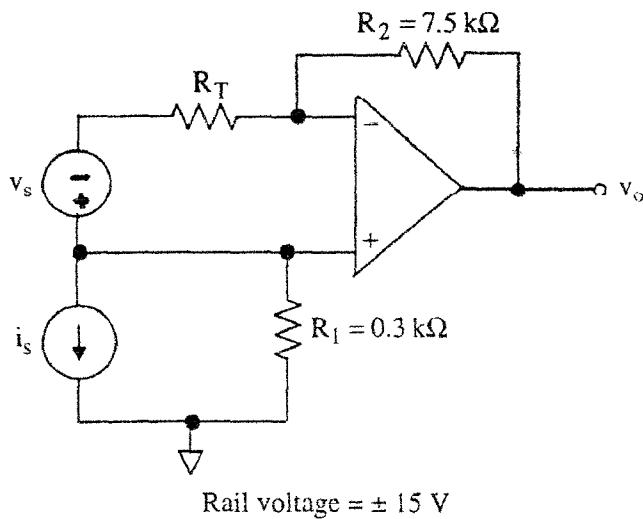
Design an electronic thermometer using the circuit diagram shown above. The voltage  $v_o$  is used to indicate temperature. Use a thermister with a resistance described by
